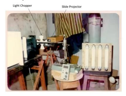
In this study, light chopper and slide projector generated particle streaks by which he could measure the velocity overshoot in flames.
